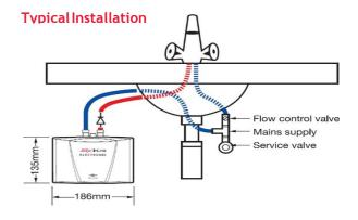
**N.B.** Zip InLine instantaneous water heating is the most efficient available, however, delivered water temperature is dependent on local incoming water temperature and supply voltage. Quoted performance assumes 12°C incoming water temperature and 230V supply.
