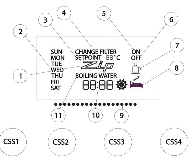
The LCD and capacitive sensor switches connect to the Controller PCB via a 4-way serial cable.
