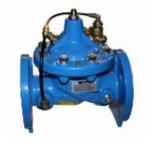
The pilot operated reducing valve reduces a higher upstream pressure to a constant lower downstream pressure. This very accurate valve is designed to operate with a minimum of maintenance. The only moving parts in the valve are the diaphragm and the stem assembly, which are guided by an exchangeable bearing in the cover and the valve seat. Easy to install and adjust.
