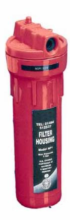
These filter housings are manufactured from glass reinforced nylon and are available with either 10" or 20" cartridges. The housing can withstand temperatures up to a maximum of 73°C. All housings are supplied complete with support brackets and a filter bowl wrench.
