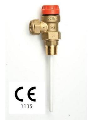
When the set conditions are reached, the valve discharges a sufficient amount of water to allow the temperature or pressure to return within the system's limits. The valves have been designed for use on unvented hot water systems.
